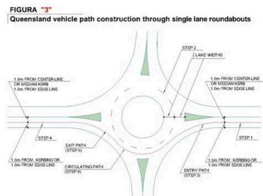
**Figure 3** provides details for a through movement
