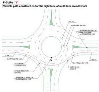
**Figure 4** provides details of the construction of vehicle paths for the right lane of multi-lane roundabouts for the through movement.
